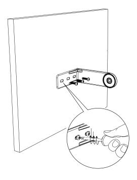
2 Synchronize the gear with surface of luminaries and leg
