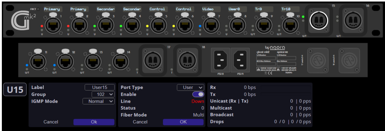
Fig.4 optional Fiber ports 15&16 can also be configurable as User ports.
