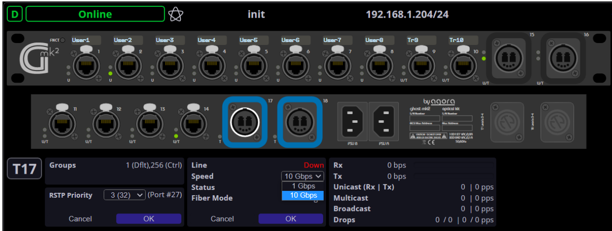
Fig.3 10Gbps optional Fiber ports can also be set to 1 Gbps speed.
