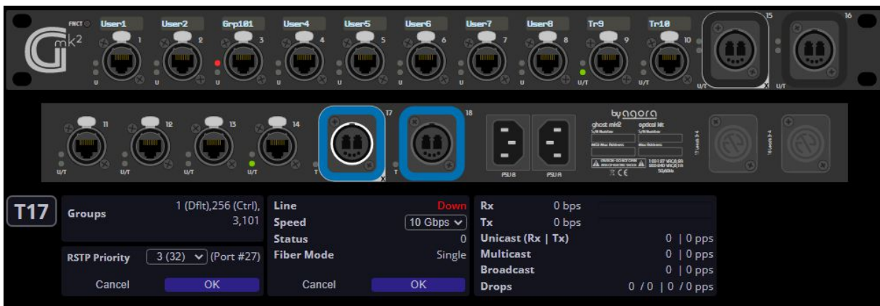
Fig.4 10Gbps optional Fiber ports can also be set to 1 Gbps speed.
