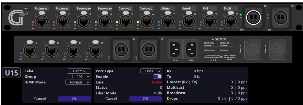
Fig.5 optional Fiber ports 15&16 can also be configurable as User ports.
