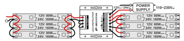
• Switch on the power supply AFTER you checked all connections.
