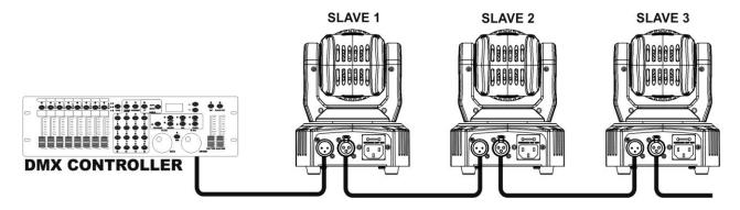
Each light effect in the chain must have its proper starting address so it knows which commands from the controller it has to decode.
