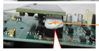
If needed, put some silicon glue on the connector to secure it.
