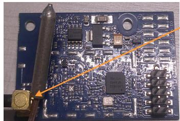
Plug the antenna in the wireless adapter board, see picture
