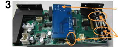
Position the WDMX module on the PCB (see picture) and insert the male pinheader in the female connector on the PCB.
