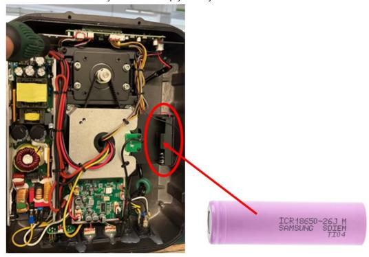
3. Insert the battery (model: 18650 \* 3,7V Li-ion) in the battery slot. Pay attention to the correct direction and polarity.
