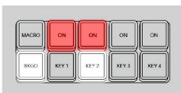
Control panel next transition buttons before transition.
