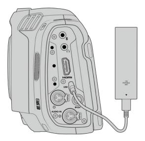
**NOTE** When a USB-C flash disk is connected to your camera, it occupies the second storage slot in your camera's operating system.
