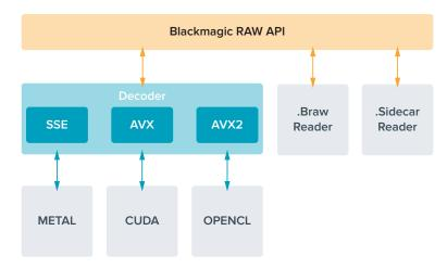
The following diagram illustrates the components of the Blackmagic RAW API:
