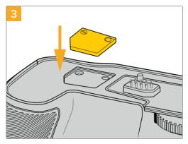
For safe storage of the contacts cover from the underside of camera, insert it into the recess on top of the battery grip and secure it in place by tightening the screw.
