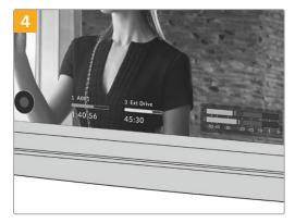
The storage information at the bottom of the LCD touchscreen will show the name and record time remaining of the detected CFexpress card.
