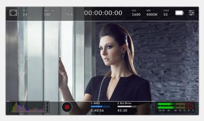
The LCD touchscreen with 2.40:1 frame guides enabled
