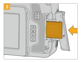
Insert the CFexpress card into the slot until you feel it lock into place. The card should insert easily without the need for excessive force. To remove a CFexpress card, gently push the card in and then release to eject it.
