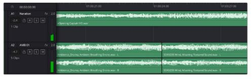
The track header on track A1 indicates a mono track with a single lane for mono audio, and the A2 track header indicates a stereo track with two lanes to accommodate stereo audio
