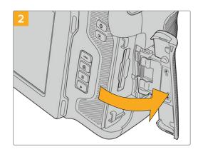
The spring loaded door opens so you can access the CFexpress card slot.
