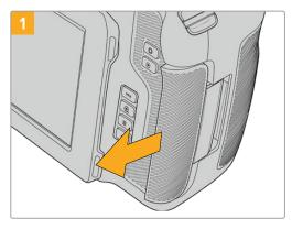
To access the CFexpress card slot, hold the camera with the LCD facing you. Slide the door on the right side towards you and then let it swing open.
