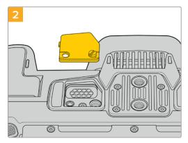
Remove the cover from the underside of the camera to reveal the electrical contacts that provide power from the battery grip.
