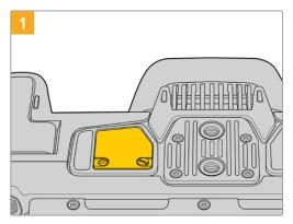
Locate the small cover on the underside the camera near the battery compartment, and loosen the screw that holds it in place.
