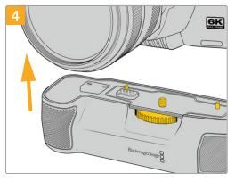
Gently push the camera grip onto the underside of your camera. The 1/4 inch screw on top of the battery grip should line up with the 1/4-20 mounting point on the base of the camera. Small pins on both sides of the 1/4 inch screw help maintain correct alignment.
