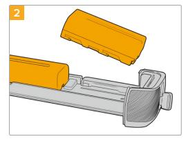
Place two NP-F570 batteries into the battery tray, being careful of their orientation, and slide them away from each other. A tab between the batteries moves up to lock the batteries into place. When you want to remove the batteries, press down on this locking tab and slide the batteries toward each other.
