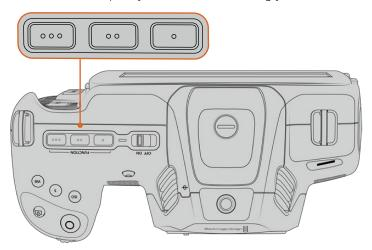
The function buttons are represented by dots and are located on the top of your camera
