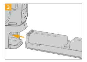
Slide the battery tray into the battery grip and turn the locking tab clockwise. It's important to note that you can continue filming while changing batteries in the battery grip if your camera is powered by an external source plugged into the DC power input.
