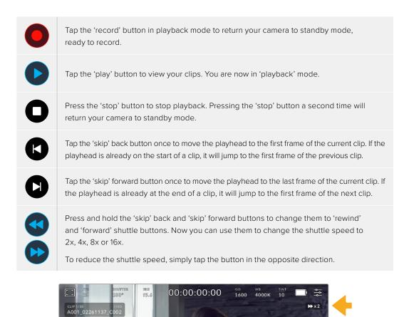
The shuttle speed indicator displays the speed and direction of footage being fast forwarded or reversed
