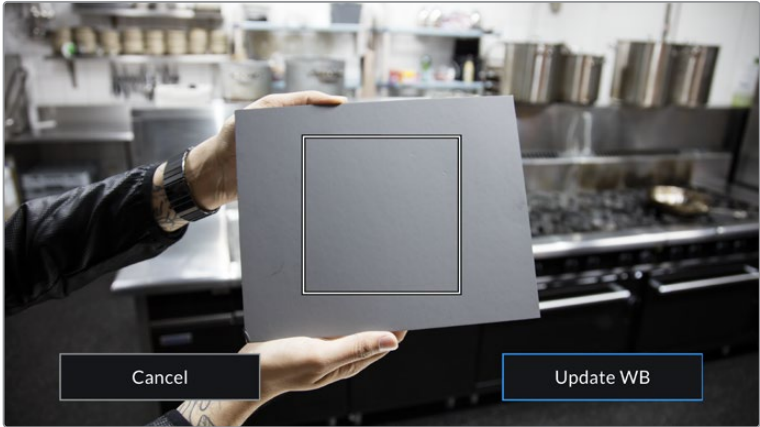
Tapping the 'AWB' icon in the white balance menu will bring up the auto white balance screen. Use this with a white or neutral grey surface to automatically set a neutral white balance
