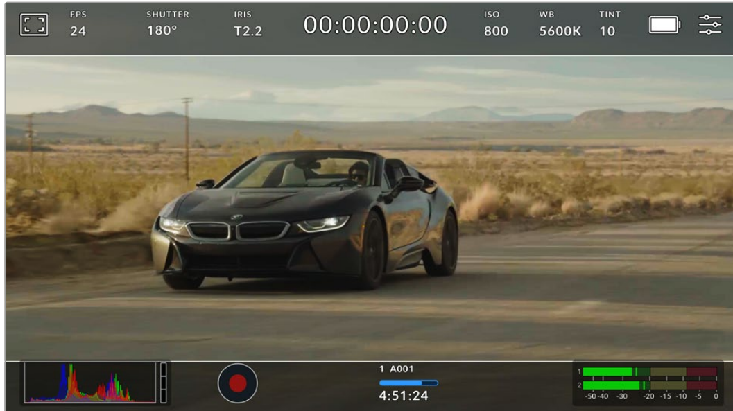
The LCD touchscreen with 2.40:1 frame guides enabled
