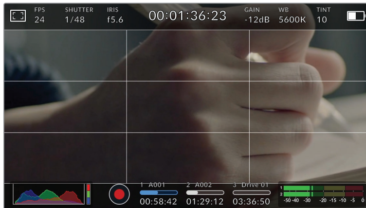
The rule of thirds grid automatically scales to any on screen frame guides
