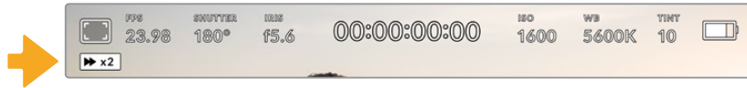
The shuttle speed indicator displays the speed and direction of footage being fast forwarded or reversed
