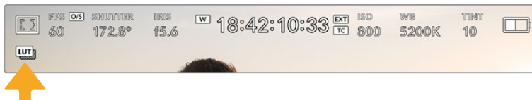
The LUT icon lets you know that you have a LUT applied to the image
