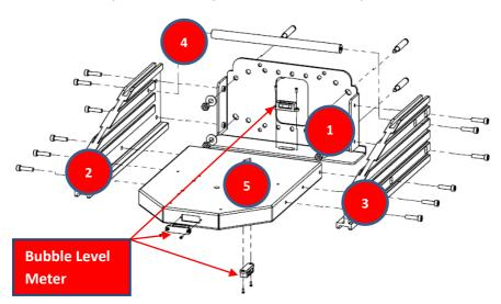
First mount a bubble level meter to the wall plate using two M2 screws. Align the wall plate with the four holes drilled in Pre-Work then use four expansion bolts to secure the wall plate. See the diagram below.
