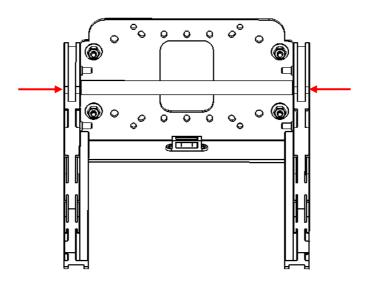
5. Use four M2 screws to mount two bubble level meters to the base plate with one in the front and one at the bottom.
