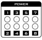
Each DC output LED indicator illuminates upon supplying power.
