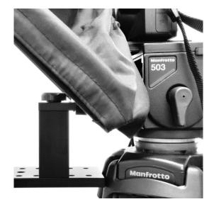
**Tip:** If you are unable to get the camera lens close enough to the TP-650 MKII due to the size of your tripod base or length of the camera lens you can reverse **item T** as shown in the image to the left. This can be achieved by undoing the two countersunk hex screws in **item B** with the hex tool, **item D1** and rotating the assembly 180 degrees.
