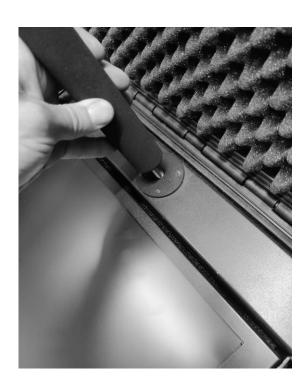
Screw on the extendable pole (Item C) onto the main TP-800 ENG hard case & chassis (Item A)
