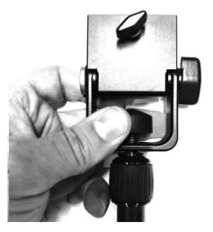
Attach the Adjustable beam splitter glass clamp (Item D) to the top of the extendable pole (Item C) using the thumb screw (Item E)
