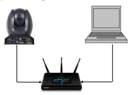
After connection has been successfully established, on your PC/laptop, use DVIP Configuration Tool to search for the camera's IP address. If you are new to DVIP, see the <u>DVIP</u> section for more descriptions of the tool.
