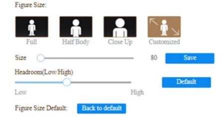
Select **Customized** if you would like to customize the tracking profile. Use the **Size** slider to adjust between 80 and 360. Use a smaller value if you would like track a closer view and use a larger value otherwise. Click the **Save** button to confirm.
