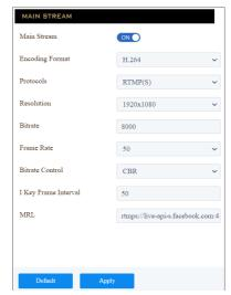
5. Click the **Apply** button to activate the RTMP video stream. Make sure both audio and video are enabled.
