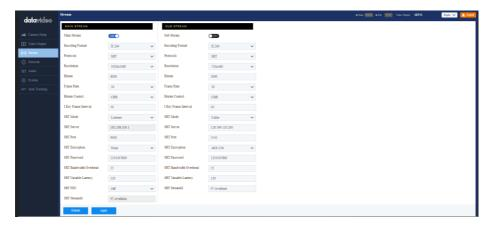
Caller and listener modes work together to establish the SRT link between source and destination devices. It is arbitrary to set one device to listener mode and the other to caller mode. Either can be the source device.
