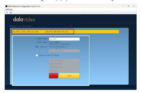
Step 4: You are allowed to change the device name in the Host Name field and modify the device's network settings accordingly. Click the Save button to confirm the change. To reset, simply click the Default button.
