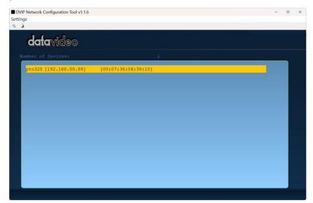
Step 3: Click one of the connected cameras to show the device information and its network settings in the pop-up window shown in the diagram below.
