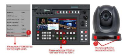
Switcher's "PGM" is set to "ON" and the "PVW" is set to "ON" (take channel 1 as an example). At this time, the tally light of the camera will be lit in green. The diagram below is a schematic diagram.
