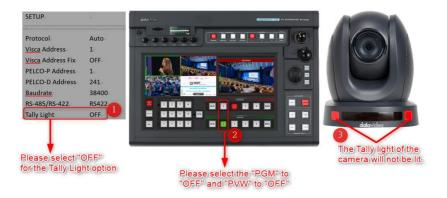
> Switcher's "PGM" is set to "OFF" and the "PVW" is set to "ON" (take channel 1 as an example). At this time, the tally light of the camera will not be lit. The diagram below is a schematic diagram.
