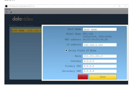
Step 4: You are allowed to change the device name in the Host Name field and modify the device's network settings accordingly. To reset, simply click the Default button.
