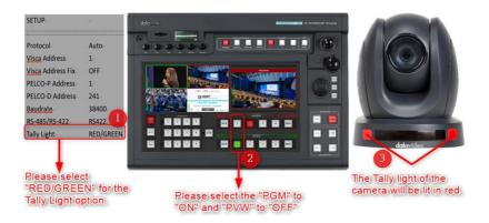
➤ Switcher's "PGM" is set to "ON" and the "PVW" is set to "ON" (take channel 1 as an example). At this time, the tally light of the camera will be lit in red. The diagram below is a schematic diagram.
