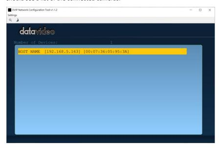
Step 3: Click one of the connected cameras (HOST NAME) to show the device information and its network settings in the pop-up window shown in the diagram below.
