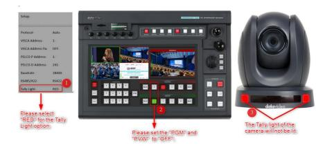
> Switcher's "PVW" is set to "ON" and the "PGM" is set to "OFF" (take channel 1 as an example). At this time, the tally light of the camera will not be lit. The diagram below is a schematic diagram.
