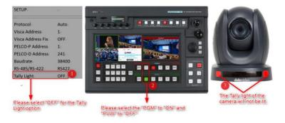
➤ Switcher's "PGM" is set to "ON" and the "PVW" is set to "ON" (take channel 1 as an example). At this time, the tally light of the camera will not be lit. The diagram below is a schematic diagram.
