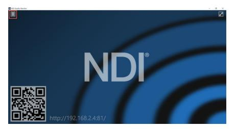
Click the PTC-140NDI camera detected by the NDI Studio Monitor to view the camera video. You can also enter the link highlighted in the red rectangle into the address bar of a web browser to view the camera video.
