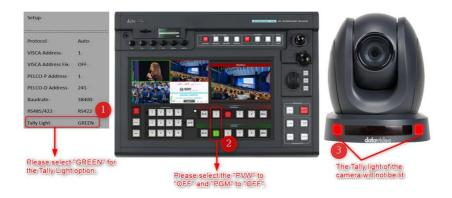
> Switcher's "PGM" is set to "OFF" and the "PVW" is set to "ON" (take channel 1 as an example). At this time, the tally light of the camera will be lit in green. The diagram below is a schematic diagram.
