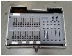
*DMX Controller The DMX Controller is used to control al TCM DMX Devices.*
