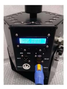
Connect the DMX cable to the DMX in connector. Connect the other end of the DMX cable to the DMX Controller.
