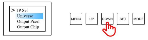
Click the SET button to enter the options, you can modify the option parameters. Click "SET" again to save, and long press "MENU" to return to the initial interface. The output of the controller port is an independent port output, and the port can carry a maximum of 680 pixels;
