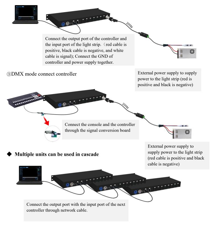
Note: When multiple controllers are cascaded, each controller IP setting cannot be the same!
