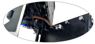
The back of the Light Matrix module is close to the cabinet to complete the magnetic fix installation.
