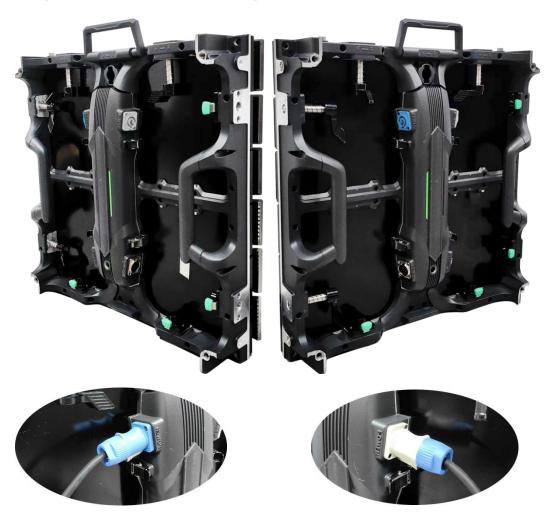
Power cable cascading: the output end of the previous cabinet is connected to the input end of the next cabinet to complete the power cascading;
