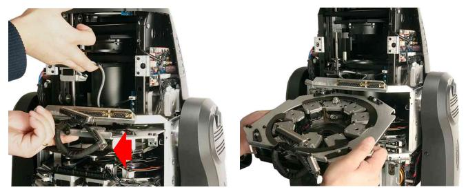
6. With the internal lens assembly lifted, carefully remove the effect module from fixture.
