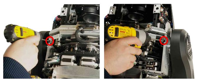
4. Remove (2x) #2 Philips screws securing the effect module.
