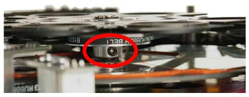
8. Loosen (2x) #2 Allen set-screws on the Static Gobo wheel gear spindle (located between the Static Gobo wheel and the Color wheel).
