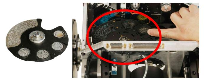
11. Carefully insert the desired Static Metal Gobos into the new Gobo/Animation wheel, making sure each of the 4 Static Metal Gobos are securely in place before installing Gobo/Animation wheel into the fixture. Reverse instructions to complete installation.
