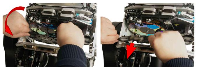
9. Because the internal lens assembly impedes the removal path of the Static Gobo wheel, disengage the TILT lock and invert the head. This will lower the internal lens assembly out and away, providing a clear path to remove the Static Gobo wheel.
