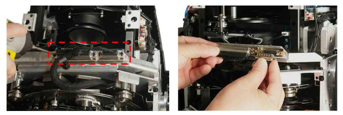
3. Remove (4x) #2 Philips screws securing 2 wire harness connectors, then carefully unplug both connectors.
