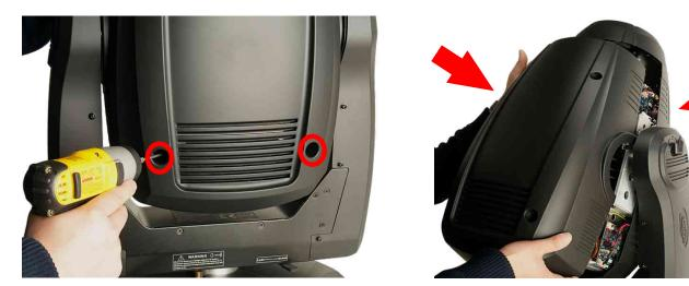
2. Remove (2x) Phillips screws securing top and bottom head panel covers, remove both covers.
