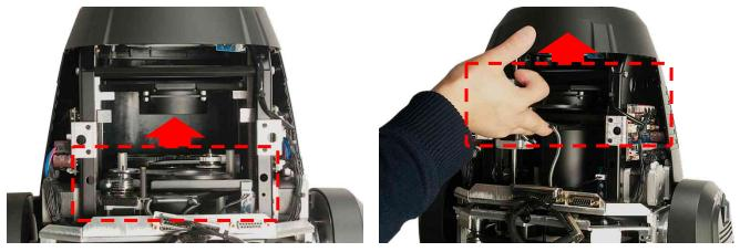
5. Because the internal lens assembly passes through the effect module tray, it needs to be lifted out and away from the effect module in order to remove it.
