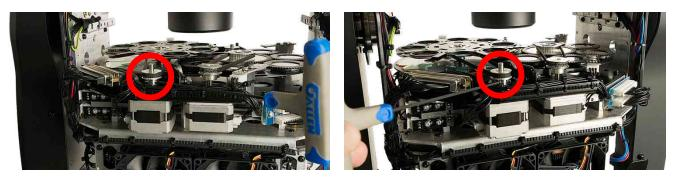
7. Loosen (2x) #2 Allen set-screws securing the belt gear spindle. This will reduce the belt tension on the Static Gobo wheel gear spindle.
