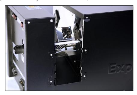
The angle block is mounted to either side of the swivel head. A sturdy metal pin can be moved freely to every angle. The X2 Wave Flamer automatically detects the position of the block, and will save it in its software. It is still recommended however, to still manually enter the preferred angles beforehand in the devices menu.
