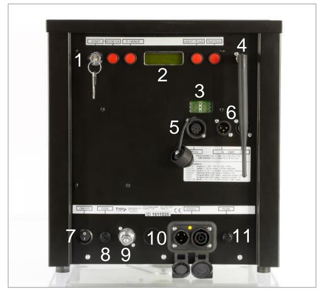
**Components of the X2 Wave Flamer** 7 1 Key switch ON/OFF switch (Power) 2 8 Fuze 12VDC Display and usage buttons 9 Status-LEDs Connector for external pumping unit 4 10 Antenna socket Power connector 100-230VAC Neutrik True-1
