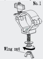
(2) Connected to the target product (Object), then tighten the wing nut.
