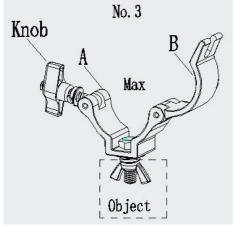
④ Fix the coupler on the pipe, be sure to tighten the knob
