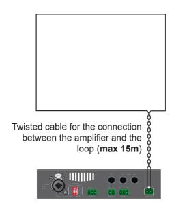
The installation consists of an electrical wire that runs through the perimeter of the room forming a loop.
