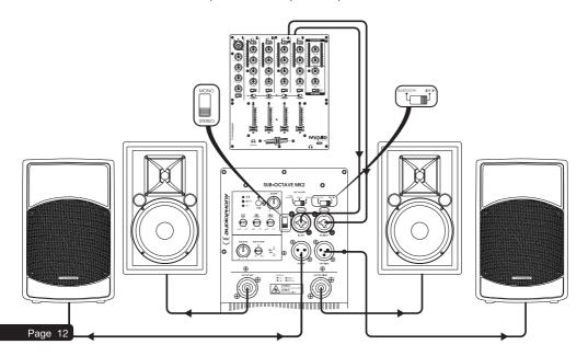
Principle 3: Mono wiring
