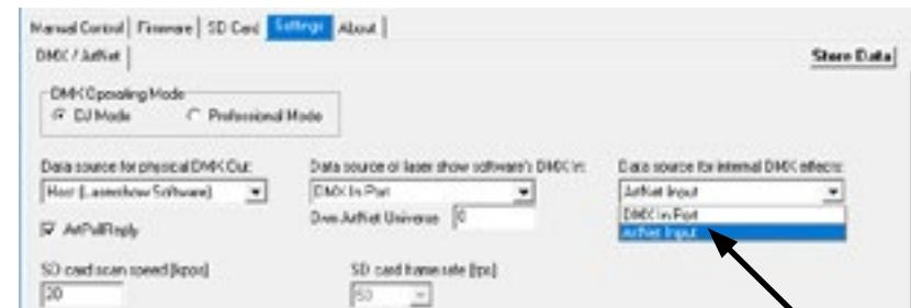
Click on ,Store Data' to save the changes. Click on ,OK' twice and wait until another window opens that asks to restart the ILDA interface. To do so, switch the laser system off and on again.
