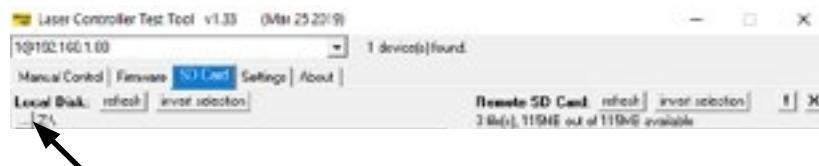
IMPORTANT: Custom laser files have to be stored in \*.ild format and must be named with a number from '000.ild' to '255.ild'. Each number represents a DMX value on the respective
