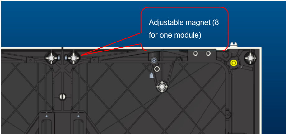
Fig 2-13 Schematic diagram of adjustable magnet
