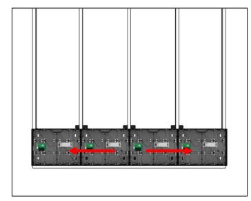
4. Observe and adjust the flatness then connect the two adjacent cabinets with screws.
