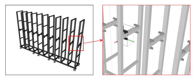
3. Select the corresponding support frames of second layer according to the size of screen, then fixed them with the first layer by screws. Repeat the previous steps to complete the assembly of second layer support frames.
