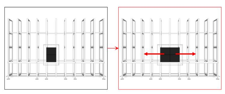
2. The crossbar will increase the ground clearance height of first layer cabinets. Then continue the **STANDARD OPERATION STEPS NO.5~8** to complete the installation.
