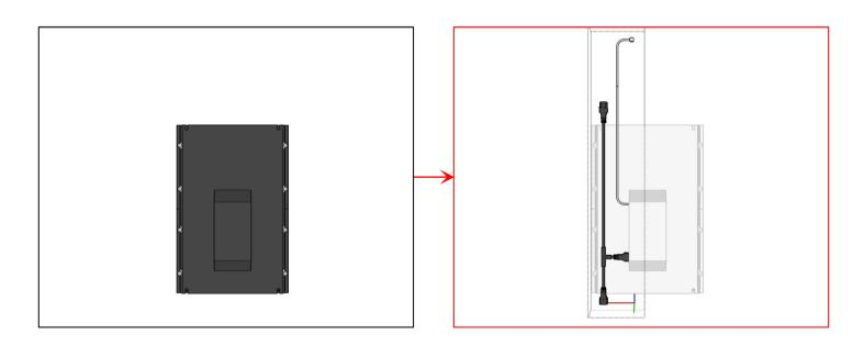
2. Connect the power cable and DATA cable on cabinets before installation. One power cable and one DATA cable on each cabinet.
