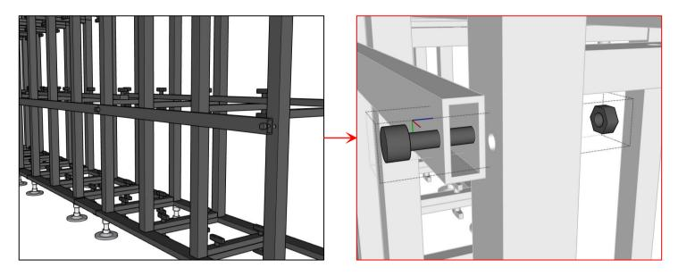
1. Select the corresponding crossbar then fixed it with bases support frames by using screws and nuts.
