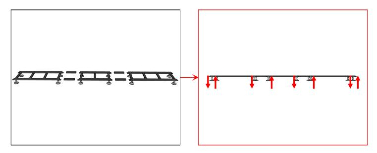
1. According to the screen size select the stand bases and connection tube, then splice them in sequence. Check and adjust the level while splicing.
