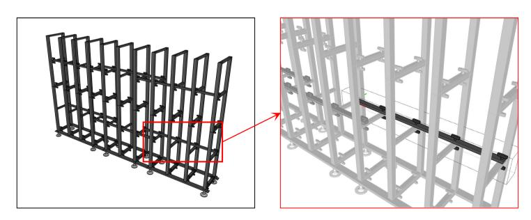
4. Place the pull rod inside the support frames, fixed it with support frames by screws & nuts.
