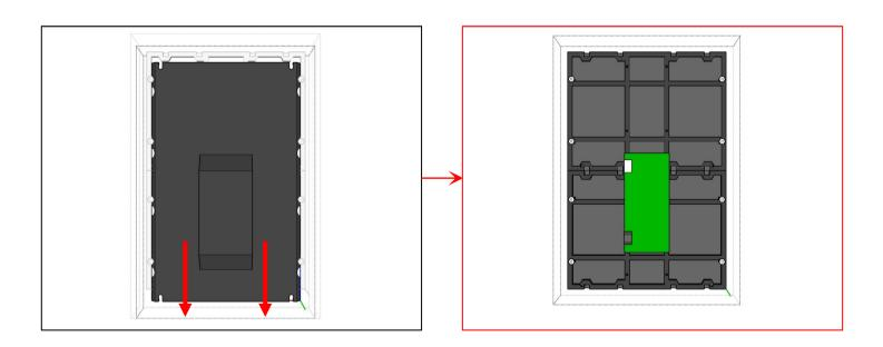
2. Slide the back cover downward then remove it to maintenance the cabinet. Release the screws to replace the module or receiving card.
