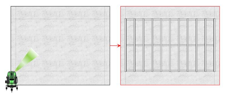
1. Measure the installation position of the screen and confirm the staring position. Keep the measuring equipment vertical and horizontal then fixed the structure to the wall.
