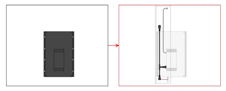
5. Connect the power cable and DATA cable on cabinets before installation. One power cable and one DATA cable on each cabinet.
