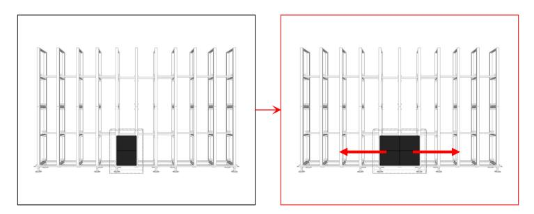
6. Place the cabinets to the beam at the bottom of structure. Recommend to install the cabinets from middle to reduce the install error.
