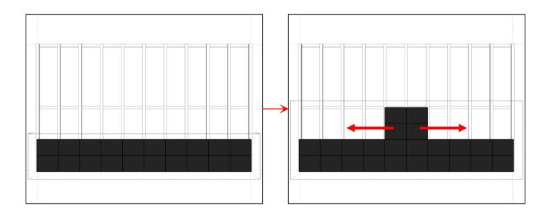
4. Repeat the previous steps to install the first layer cabinets. Place the second layer cabinets on the first layer cabinets. Observe and adjust the flatness and connect the cables while installing.
