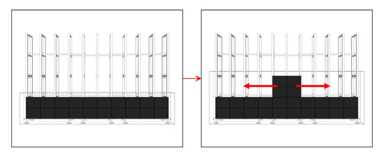
7. Repeat the previous steps to install the first layer cabinets. Place the second layer cabinets on the first layer cabinets. Observe and adjust the flatness and connect the cables while installing.
