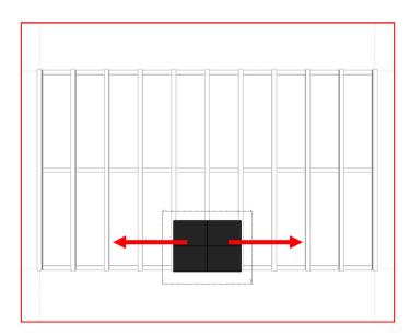
3. Place the cabinets to the beam at the bottom of structure. Recommend to install the cabinets from middle to reduce the install error.
