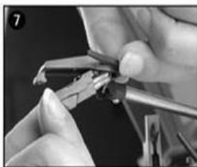
3 separate the cartridge from the socket lightly.
