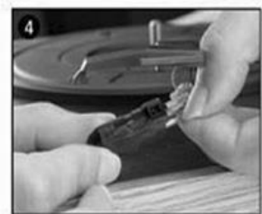
4 take off the audio-line from the cartridges completely.
