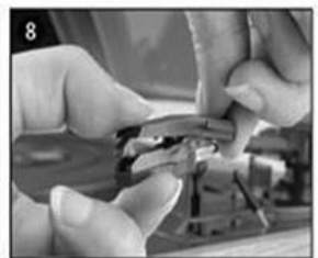
4 take off the audio-line from the cartridges completely.
