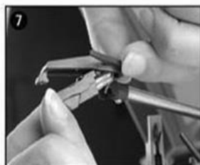
3 separate the cartridge from the socket lightly.
