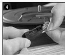
4 take off the audio-line from the cartridges completely.
