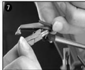
3 separate the cartridge from the socket lightly.
