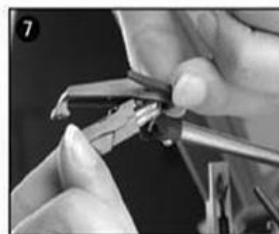
3 separate the cartridge from the socket lightly.
