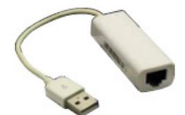
\*Prepare a RJ45/USB converters if necessary
