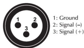
DMX-input XLR mounting-plug:
