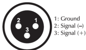
DMX-output XLR mounting-socket:
