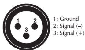
DMX-input XLR mounting-plug:
