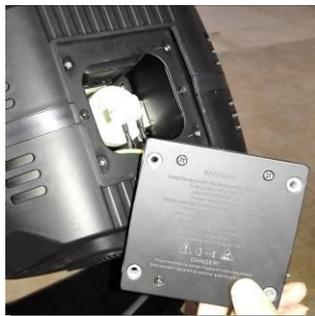
3. One hand press the lamp holder, another hand hold the lamp, and pull out the wires (picture 3,4)
