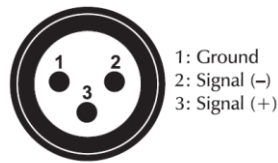
DMX-input XLR mounting-plug:
