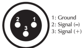
DMX-output XLR mounting-socket:
