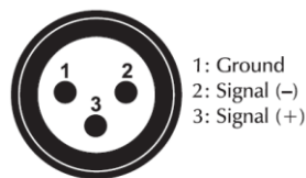
DMX-input XLR mounting-plug:
