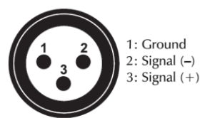
DMX-input XLR mounting-plug:
