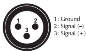
DMX-input XLR mounting-plug:
