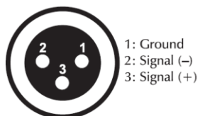
DMX-output XLR mounting-socket:
