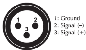
DMX-input XLR mounting-plug:
