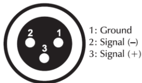
DMX-output XLR mounting-socket:
