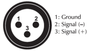
DMX-input XLR mounting-plug:
