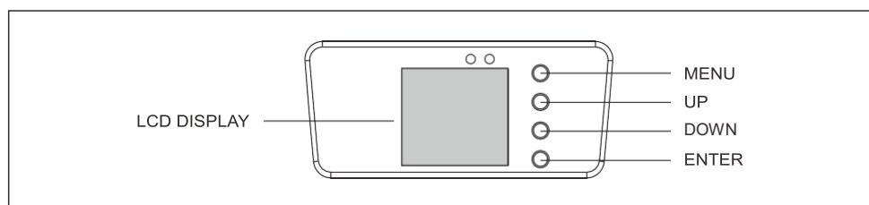
Access the menu directly by pressing the **Menu** key and move through the menus with the **UP & DOWN** keys. Press the **ENTER** key to confirm your choices and values.
