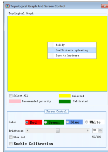
Fig. 4-21 Uploading calibration coefficients via topological graph
