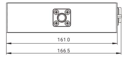
Tolerance: ±0.3 Unit: mm
