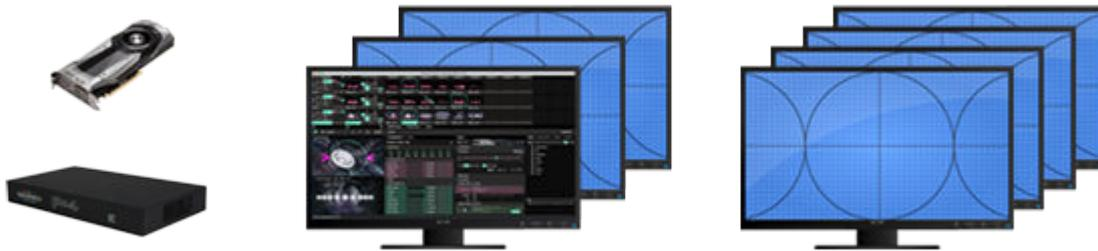
This is the next best thing. By using extenders like the Datapath Fx4, you can extend a single port to multiple outputs. Resolume will think your output just got a lot bigger, so all rendering still goes over your main GPU without any additional performance hits.
