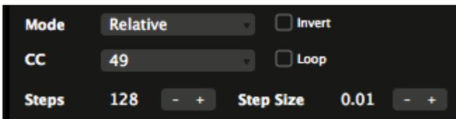
Some rotary knobs don't send out fixed values between 0 on their left side and 127 on their right side. Instead of coming to a stop on each end, you can twist them endlessly in both directions, and they will keep sending out different values. For instance, the APC40 MK1 has a relative rotary above the master fader. The MK2 even has two, the second one is placed on the top right next to the Tap button.
