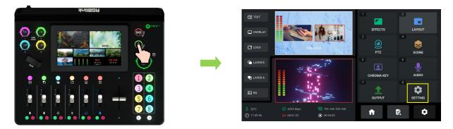
Tap [SETTING] or push Button 8 to enter Setting Interface. You can also access to Setting Interface
