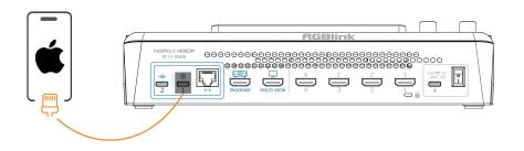
2) Then the 'Trust This Computer' alert message will appear on your device. Tap 'Trust' on your device and do as followings: Open 'Settings' > Select 'Personal Hotspot' > Enter 'WLAN Password' > Turn on 'Allow Others to Join' .
