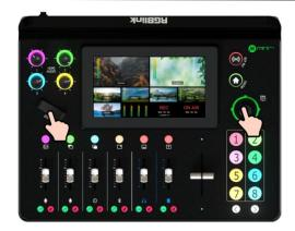
4. Long press Layer A/Layer B/Logo/Overlay Button to enter Layout Selection Interface. Or you can tap LAYOUT icon in MENU or push Button 2 to enter Layout Selection Interface. RGBlink offers 7 layout options. If the Layout [6] is selected, use the Adjuster to achieve a better
