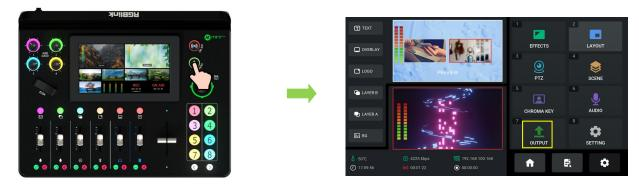
Tap **Stream** in **[**OUTPUT**]** menu to enter streaming configuration interface.
