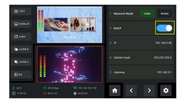
Static (set IP freely by yourself): Turn off DHCP to manually set IP address. Then click "Enter" to conform your setting.
