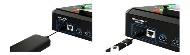
Insert a U disk or SSD to USB port labeled number 1. Before recording, format the U-disk or SSD
