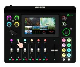
2. Push Button 1~4 on the front panel to select the input.
