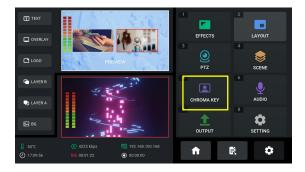
5. Users can choose ON or OFF to enable or disable Chroma Key (off by default). Select the background color which is default in green to be removed and make adjustments according to application.
