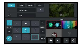
mini-mx supports simultaneous control of up to four cameras.
