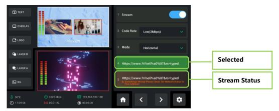
**mini-mx supports streaming up to 2 platforms at the same time**. Turn on Stream on the interface or push ON AIR Button on the front panel to start streaming.
