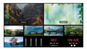
Users can switch screen mode and select HDMI output resolution by pressing [OUTPUT] on the main menu.
