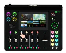
2. Push Button 1~4 on the front panel to select the input.
