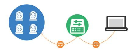
4) Connect mini-mx and camera to the switch via Ethernet cables (It is recommended to use
