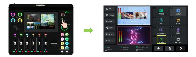
Tap [OUTPUT] in MENU or push Button 7 to set parameters for video output.
