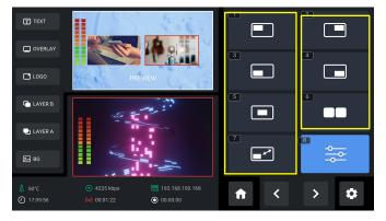
5. Click Option **[8]** Advanced Setting to do more specific parameter settings for layer cropping and scaling. As shown in the figures below, use joystick to choose item and then do settings by using slide bar or adjuster.
