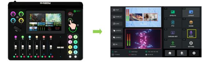
Tap 【AUDIO】 or push Button 6 to enter the Audio Management Interface. You can also access to the following interface by single click/double click/long press on Audio Monitoring Area on Main Interface.
