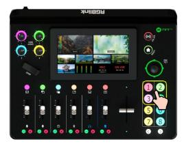
3. Use the Adjuster on the front panel for zoom-in and zoom-out of Layer A and the Joystick to quickly adjust horizontal and vertical position. Push joystick to full screen mode, then push it again to restore to the size and position last set.
