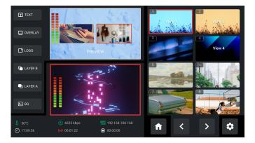
2) mini-mx allows user to save 16 presets in total to the corresponding View 1~16. Long press Preview Window in Editing Interface or Main Interface, and you can choose whether to form a static picture of the current scene and save it or not. mini-mx can save the formed picture to
