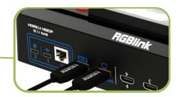
The default output of MULTI-VIEW port is multi-screen Preview view, so user can see the audio and video conditions of all input signal sources, check current status of each function of mini-mx and see the Preview view.
