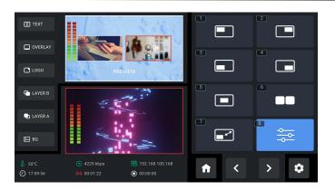
4. mini-mx supports matting, that is, removing the pure color background and overlaying it on another signal to realize the application of virtual reality. Push MENU Button to enter Main Menu, tap [CHROMA KEY] in MENU or push Button 5 to enter the setting interface.
