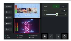
mini-edge **defaults to T-Bar Mode**. Users can also switch to CUT Mode and then use Button 1~5 on the operation board to switch inputs.
