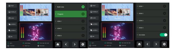
Default to be Multi-view preview, which can be switched to Program, Test Pattern or 1~4 HDMI inputs for various applications.
