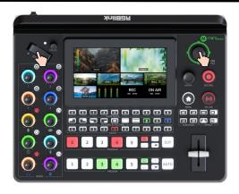
4. The user can gain access to Layout Interface through the following methods:.Long press Layer A or Layer B button. Or you can push MENU button to enter menu interface. Use ENTER knob to move the cursor to LAYOUT icon, press ENTER knob again to enter. Select required layout for Layer A and place it on the background.
