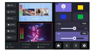
Check the background color required and then use 5-direction joystick to shift options between Max, Min and Margin. Max defaults to 1232, Min defaults to 560, Margin defaults to 200.
