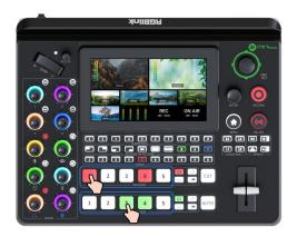
3. Use the toggle on the control panel for layer zoom-in and zoom-out and the joystick to set the position for more detailed adjustment.
