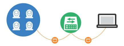
4) Connect mini-edge and camera to the switch via Ethernet cables (It is recommended to use RGBlink CAT6 cable with order code as 940-0001-00-11-0). Then use mini-edge for PTZ control.
