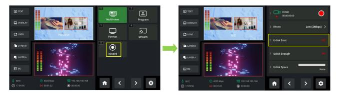
After USB disk is inserted, please do as follows: Set the file system to exFAT and the size of allocation unit to 128kb > Disk formatting > Confirm to format disk.
