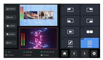
Rotate ENTER knob to move the cursor to SCALE or CROP icon, press ENTER knob again to do more specific parameter settings for layer cropping and scaling.
