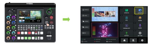
PIP layout allows multiple windows to be displayed simultaneously on a single screen, offering users a perfect platform to check multiple video contents at the same time. The PGM Program is
