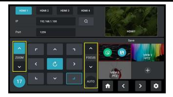
Use Joystick to adjust position of camera.
