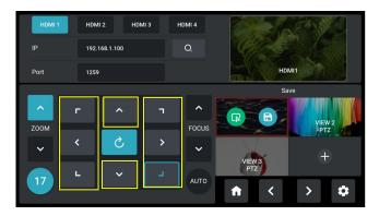
As shown in the figure below, the number displayed indicates the rotation speed of the camera.
