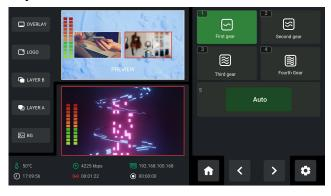
In the fan control interface, four levels of fan speed for users to choose from. Choose **Auto** to achieve automatic adjustment of the fan speed.
