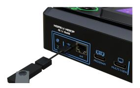
Insert a U disk to USB port labeled number 1. Before recording, format the U-disk first.
