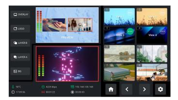
mini-edge allows user to save 10 presets in total to the corresponding View 1~10. If the selected window does not contain a preset, press ENTER knob to choose whether to form a static picture of the current scene and save it. If the window has stored a preset, press ENTER knob to choose whether to delete or overwrite.
