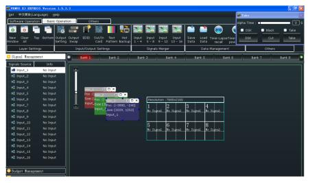
**Paste Layer:** Put the mouse on the window to be copied, right click the mouse, select "Copy Layer", then right click in output screen zone of controlling software, and select "paste Layer".
