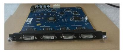
② For the joined PCB input module with CVBS, HDMI, VGA, USB or SDI interface, fix the input module on the plate with 2 M3\*4 flat screws and 2 M3\*4 round head screws.
