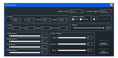
Full or Close Window: Click the icon "I" at the upper right corner to full cell and click the icon "I" at the upper right corner to full screen. Or put the mouse on the window to be adjusted, right click the mouse, select the "Full Cell" or "Full Screen".
