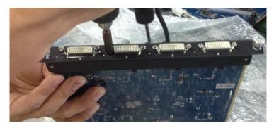
4. Push the input modules into the device along the slide rail, and screw the captive screws, as shown in figure:
