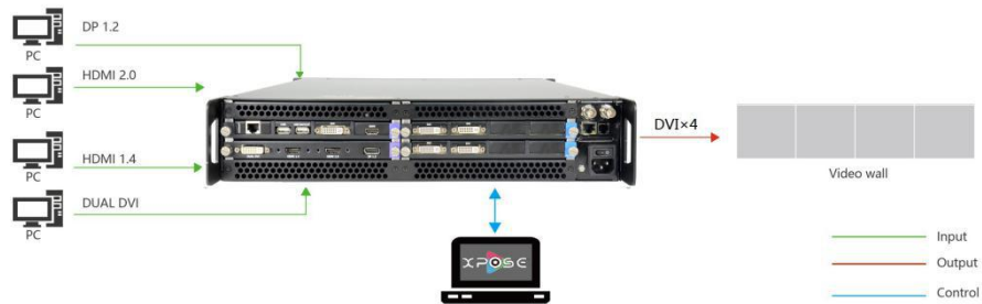
FLEX4ML System Connection Diagram
